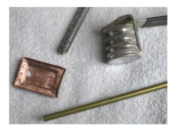
Note : I used to punch a little bit the copper sheet around the hole by means of a very coarse puncher visible on the top of the picture. It is a piece of round steel bar of which the extremity has been formed as a cone by means of a grinding machine. I put the copper part on a piece of soft wood, and with the puncher I deform it so as to put the pipe end not too close to the future diaphragm. This is not a must, but it could help.
