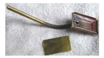
Then lay a very thin filler string along the angles of the folded sides, and put the diaphragm above. Fold completely the sides by means of pliers or vice to pinch the diaphragm all around.
