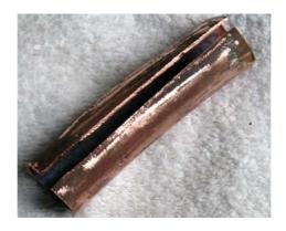
Widen the opening by means of two screw drivers, then by means of pliers. If the pipe has been annealed properly, this should be very easy. Put the unrolled pipe on a flat support and hammer it lightly to flatten it. Here is the result.
