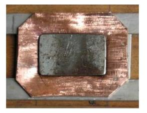
Then, with pliers or vice, fold the sides, at approximately 90 degrees in a first step. And, with the drilling machine, drill a hole to introduce the pipe (or the pipes. When there are two pipes, filling the engine with water is easier once the engine is finished).
