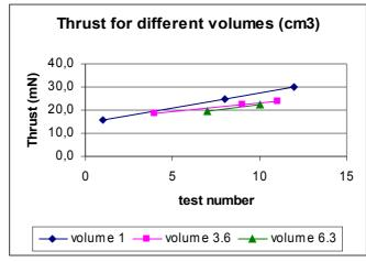
From these graphs we get confirmation of "rumors" or assumptions: for a given surface of the heating chamber, the thrust increases when the volume decreases.
