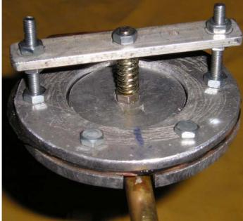
A spring has been added. At rest the spring is compressed. The compression force is adjusted by means of the central nut. The diaphragm is in a fixed position adjustable by means of the lateral nuts on both sides.
