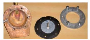
This diaphragm (in the middle of the picture) is made of rubber with a rigid part in the middle. A screw at the centre allows to adjusting the vertical position of the diaphragm, i.e. the volume.
