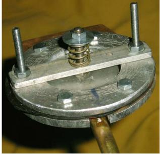
Another spring (softer) has been used. At rest the spring is compressed. The compression force is adjusted by means of the central nut. The diaphragm is in a fixed position. Its lower nut is against the transverse bar. When the pressure is low enough to develop a force bigger than the spring one, the screw with its central nut goes down and the movement is visible (and audible).
