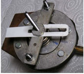
Note: At low pressures the accuracy is not very good because the diaphragm which is made of rubber has also a spring effect. We recorded the following data:
