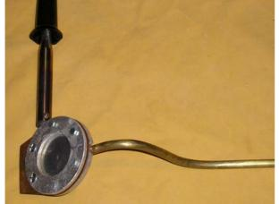
On this picture the soldering iron visible on the left has been modified. It is fixed to the steam drum. At the bottom, towards the right side is the single pipe.
