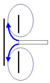
Such a screen doesn't prevent vortexes, but they are large rand the water which comes again towards the target has lost most of its velocity.
