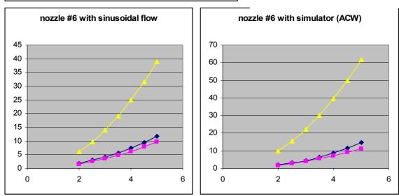
With the nozzle#6, like with the nozzle #3, we find again a measured thrust bigger than the theoretical mean value.
