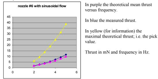
The thrust measuring test bench indicates <u>always</u> (we ran approx hundred tests) a thrust that is bigger (by 10 to 40%) than the theoretical mean value. This could be caused by at least two phenomena:
