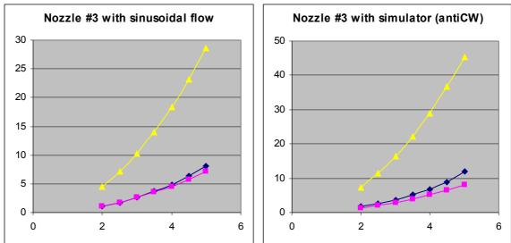
The blue curve shows the measured thrust. The magenta one shows the calculated mean value. Both curves should be identical. The yellow curve shows the pick value of the thrust. For the simulator, the graph displays what we got in the anticlockwise running. In the other way the curves are similar. They are not displayed to limit the size of this report. Then we did the same with the nozzle #10.
