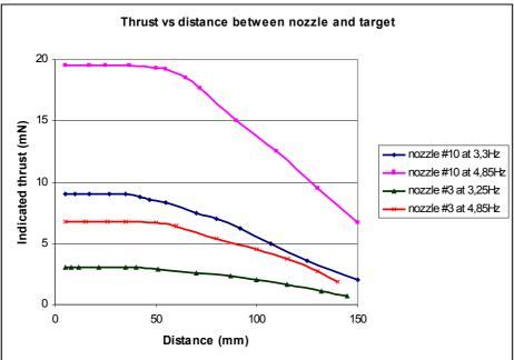
One can see that up to 40mm there is no decrease of the indicated thrust. As all our measurements were done with a distance between 10 and 15mm they are not erroneous because of the distance.
