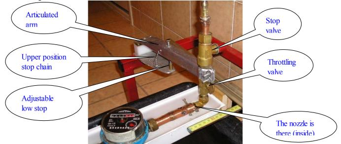
The (white) tank is horizontal and full, overflowing all along both sides. (No recirculation)
