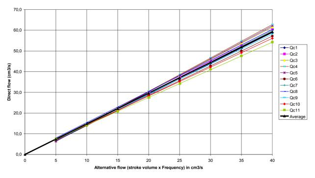
Direct flow which would give the same result as a reciprocating one (for various nozzles).
