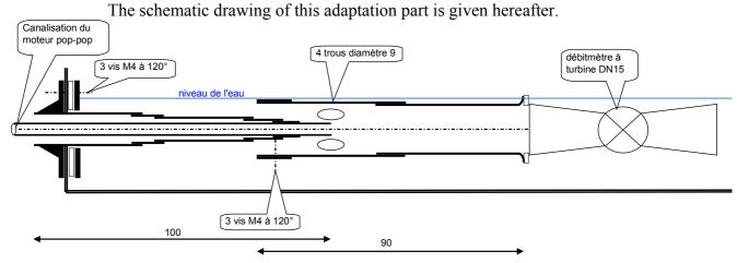
It is the part which is 90mm long. The part which is on the left will be mainly used later with pop-pop engines. The immersed part of the pipe is very short, and the pipe is close to horizontal as it is generally in pop-pop boats.
