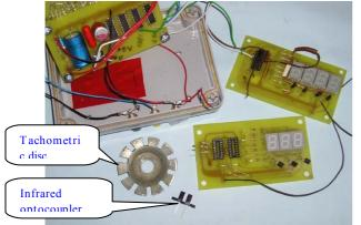
The first tachometry Much energy spent for poor results
