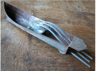
It is fitted with three pipes. This is not new. But what is unusual is the fact the diaphragm is on the bottom side.
