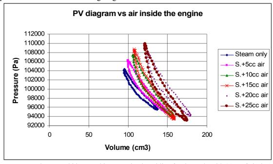
Note: In order not to hide something I used a dotted line for the cycle with 20cc of air, but this one is not as expected because it was recorded after a burn-out.
