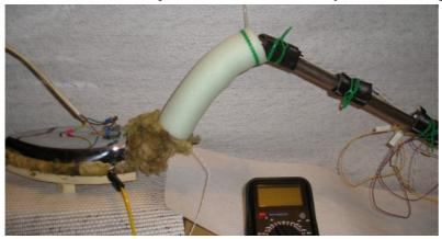
View of the engine isolated and provided with measuring instruments. The yellow wire is the one of a thermocouple measuring the copper pipe temperature. The grey one going out of the rock wool is the one of a thermocouple measuring the temperature of the boiler copper. The 3 black polystyrene sleeves cover PTC type temperature probes. This is a partial view of the engine. Totally there are 7
