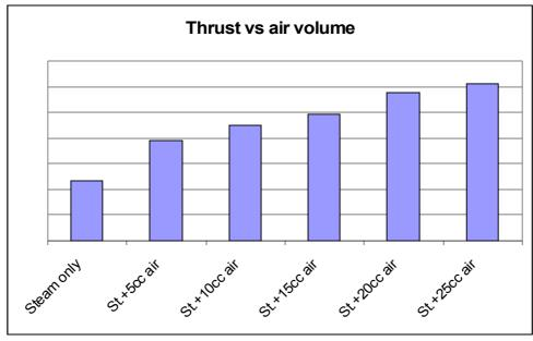
Note: for this engine 25cc of air is the upper limit. Above it, the engine stops.
