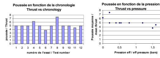
The pressure was measured with accuracy (approx +/-0.1b). For the thrust it was more difficult because I couldn't damp the mobile (target and mirror) located inside the bowl. For the accuracy I would say +/-1.5mN.
