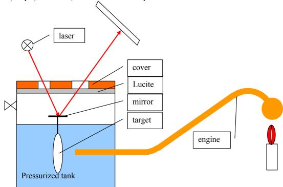
Main components from the left to the right: laser emitter, test tank (stainless steel bowl
