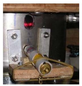
On the next release of the test bench I used a Lucite window that I had to curve as the bowl is. Due to that bending, the narrow laser beam sent by the emitter (a laser pointer, yellow on the photo) became a flat beam (visible on the upper window of the bowl).
