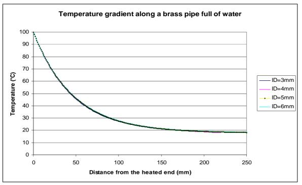
Then, for a given material I studied the temperature gradient for different pipe diameters. An example is displayed hereafter for brass pipes of thickness 0.5mm.
