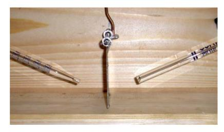
Note: On both sides the conditions were assumed to be the same but couldn't be guaranteed identical, therefore several tests were run. The drums (shortened test tubes) were interchanged to eliminate any possible volume difference, and several candles were burnt. Every time the thrust was slightly higher on the convergent nozzle side. Really slightly higher. This test was just a game. We think that a bigger difference could have been measured by using a not so narrow nozzle.
