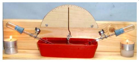
On my left hand side a pop-pop engine. On my right hand side another one. Same volume  $(4\text{cm}^3)$ , same pipe diameter (3.85mm) and length (145mm). In between: a thrust measuring device.
