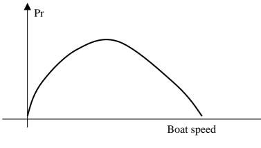
L The mechanical power propelling the boat (Pr=restituted power) is the product of the thrust T by the boat speed. It is null at bollard conditions, increases with the speed, goes to a maximum, and then decreases and becomes null (for the same speed as for the thrust).
