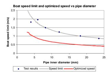
This graph set as evident the fact the speed of a boat propelled by a pop-pop engine is slow. Furthermore, it decreases when the size of the engine increases. Several small engines are preferable to a single big one.
