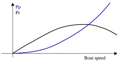
The engine/hull adaptation is good when the curves are crossing each other as far as possible from the origin, and where the restituted power is close to the maximum.
