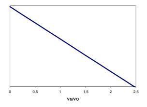
Hence, for a given pop-pop engine ( $v_0$  or C, F and d known) we see that the thrust decreases linearly when the boat velocity increases. The thrust versus  $V_b/v_0$  can be represented on a graph.
