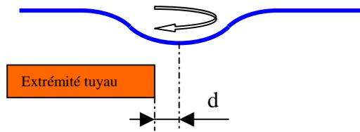
A small basin was created at the water free surface. Its centre was approximately 1.5mm ahead of the pipe. The water was rotating clockwise. (We are in the northern hemisphere).
