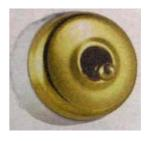
For the chamber I used the cover of an old switch. Diaphragm diameter 54mm.
