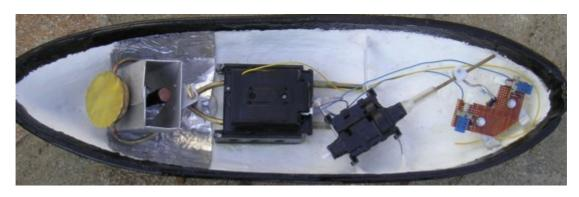
From fore to aft one can see the motor with its diaphragm, the chimney, the control unit (square black box), the (black) steering motor and the (blue) limit switches.
