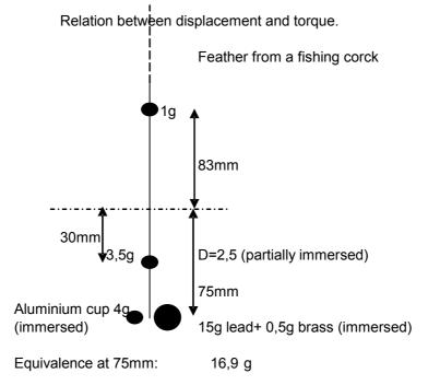
The mobile part acts as a pendulum of length 75mm and mass 16.9g. Torque = T x 75
