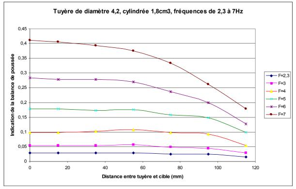
This graph shows the needle deviation versus distance for frequencies 2.3 to 7Hz. Stroke volume: 1.8 cm3. Nozzle diameter: 4.2 mm.
