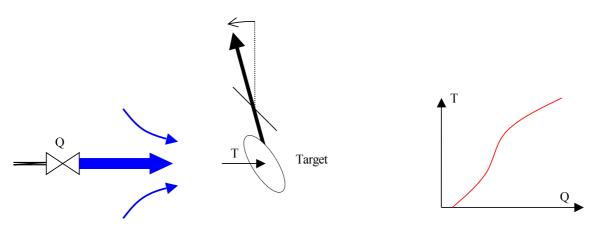
The thrust is not measured directly. In fact it is the deviation of the needle which is measured, but the torque needed to cause this deviation is known. See annex 2.
