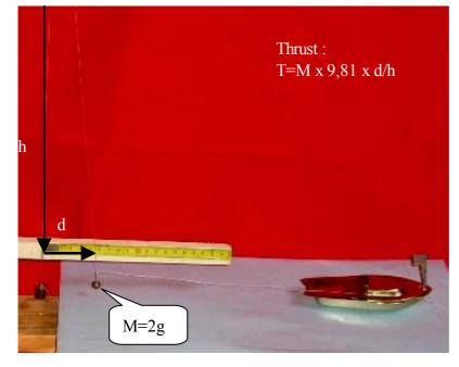
Next, we came back to a classic force equilibrium followed by a simple calculation. Two pieces of sewing thread, two masses, one of them well known, (the other one being only used for the reference plumb line) and a graduated ruler suffice. However, the forces exerted by a pop-pop engine are so weak that though a minute mass is used, the string must be long and the problems of instability exist.
