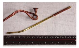
The other engine is a model of simplicity. It is made of a copper pipe 8x1 (the heated part) prolonged by a brass pipe 6x0.5. This engine worked for hours.
