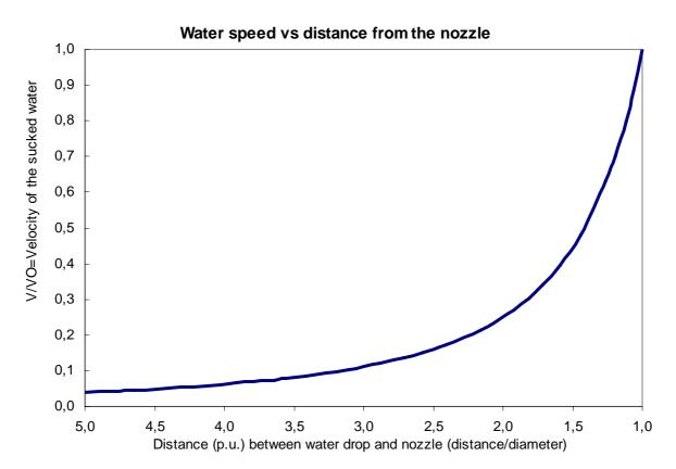
Looking at this graph allows to seeing that the velocity increases rapidly when the water drop approaches the nozzle. It also shows that for instance at a distance of only three times the nozzle diameter the velocity is approximately ten times less than the one at the nozzle end.
